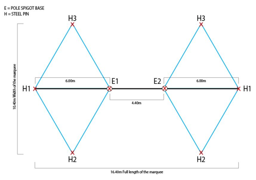
Figure 02: Layout plan – steps of spigot and peg placement
